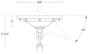
Note: This canopy requires attachment supplemental to the junction box and includes a linkage to function as a hang straight. It can be used on slopes in excess of 45°.
